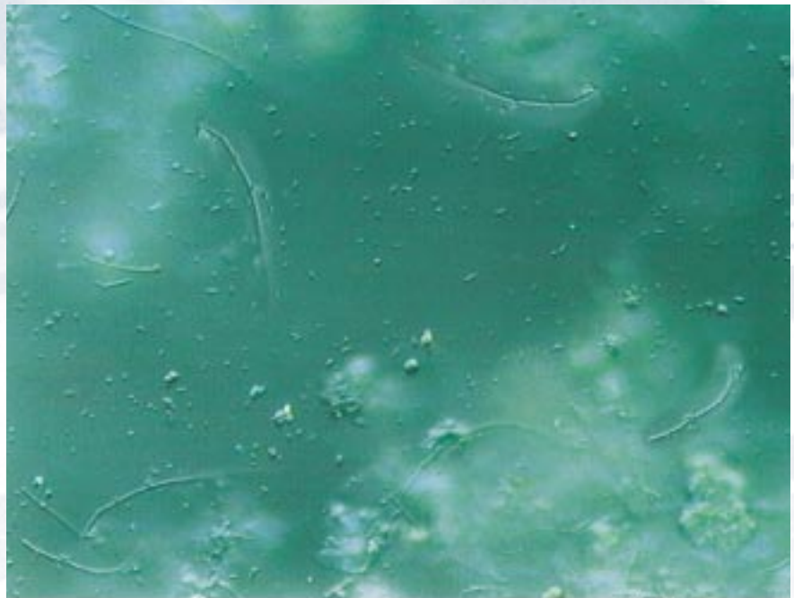
Weakly structured flocs caused by an inadequate supply of oxygen in a brewery's waste water treatment plant
