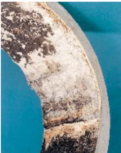
Corrosion damage on a pressure pipe
