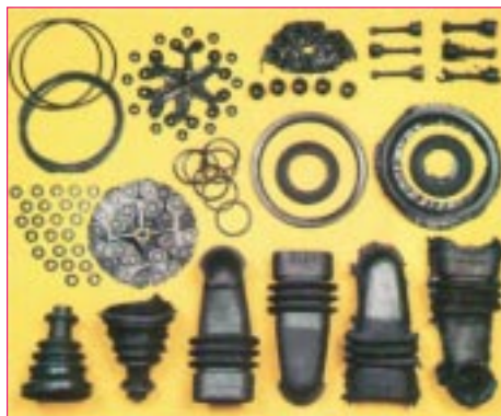
Parts before and after deflashing by a troughed belt jet deflashing machine (model MSA) or a drum jet deflashing machine (model TSA)
