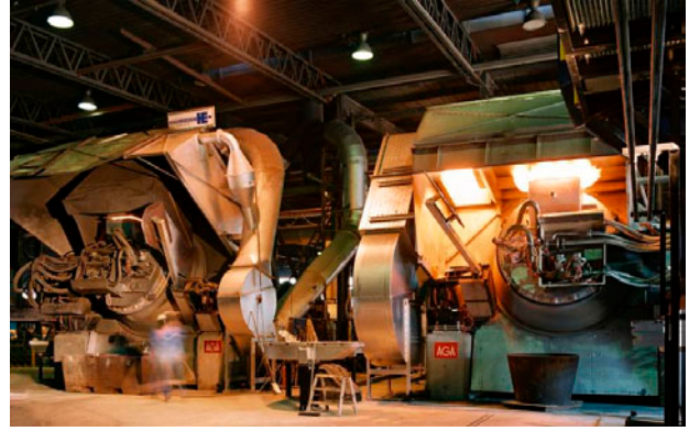
Fig. 4: Two tilt able rotary furnaces for low and ultra low salt recycling (URTF at STENA Aluminium) with oxy-fuel burners and oxygen lances (WASTOX ® ) for recycling of aluminium scraps.
