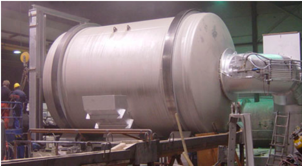
Fig. 3: Typical fix-axis rotary salt furnace (double pass) with oxy-fuel burner and oxygen lance (WASTOX ® ) for recycling of scraps in a rotary salt process.
