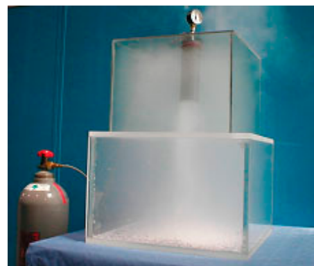
Fig. 7: Model of the furnace with functioning \text{CO}_2 -snow technique to analyse different fillings of the furnace.
