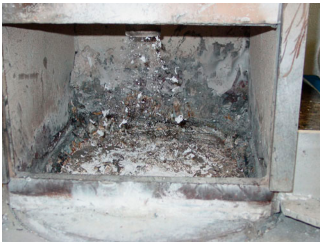
Fig. 8: CO 2 -snow falls on top of the surface of the liquid magnesium and protects the metal from oxidation.
