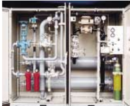
View of a membrane plant with a capacity of 150 Nm 3 /h nitrogen
